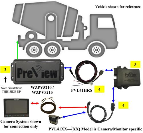
**Wire Connections Wiring Diagram**
