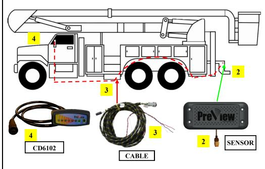
Wire Connections Wiring Diagram
