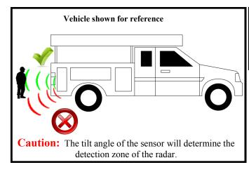
The PreView® system is a blind spot collision warning system designed to supplement other safety practices and/or devices. The machine operator is always the first line of defense when safely operating a vehicle.
