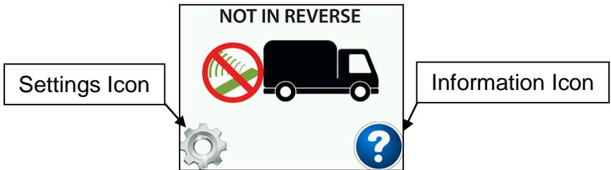
This screen allows access to the system settings and provides display information.
