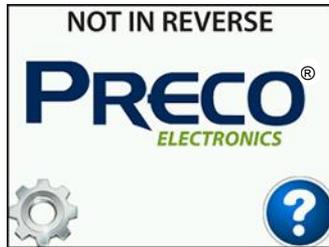
A couple seconds after power up, the PRECO Electronics® logo will change to an image depicting a truck that is not reversing (Figure 2.2). When the machine is placed into reverse and the system becomes active the screen will change to the “Active Screen”.
