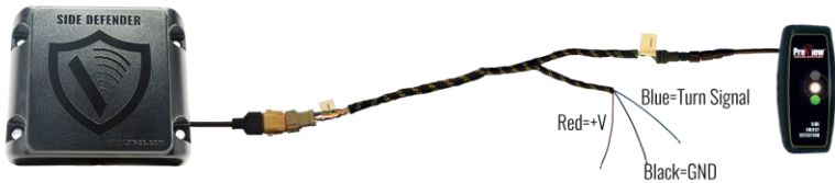
Figure 4. Wiring Connections
