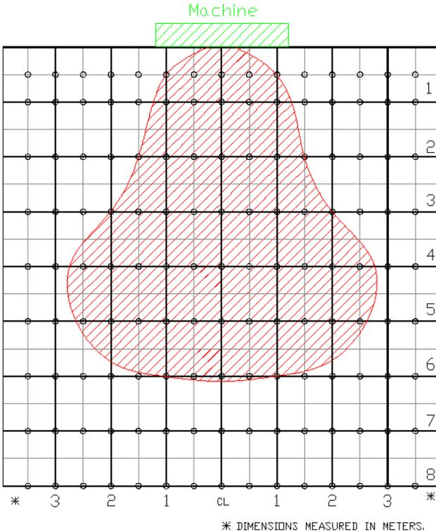
Single WorkSight sensor as observed with human target. Sensor was mounted perpendicular approx 40" from ground.
